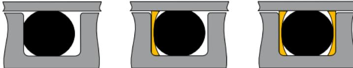
Parbak® Back-up rings prevent extrusion in high-pressure applications, help to maintain the lubricant film and thus prolong the service life of O-Rings.
