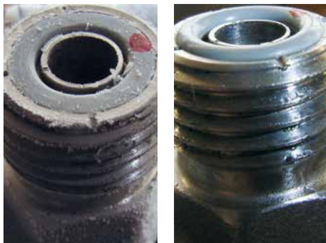
a) Frozen TPU O-ring b) Thawed TPU O-ring
